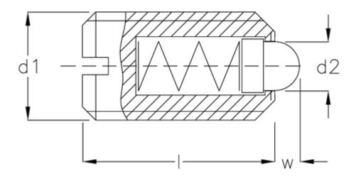
$\begin{array}{ll} d1 & = M20 \\ d2 & = 10.0 \\ Length I & = 30 \\ Spring pressure N bottom = 81.0 \\ Spring pressure N top & = 39.0 \\ W & = 6.5 \end{array}$
